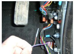
right footwell. This is a 16 pin black/red connector, C2249 (the lower section) is part of the navigation loom and contains male pins that join into the female plug socket C2247 from where the wires then go on up and back to the fuse box area.
