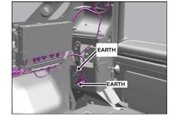
After closely studying the wiring diagrams it became clear that the RSE Module & DVD Changer should take their power from the ICE navigation loom connector C2247/C2249 located in the front
