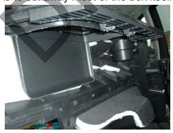
sense. Just pay close attention to the left hand side of the RSE module which needs a small additional piece removed in order for the panel to locate correctly as it sits higher than the DVD but when the hinged lid is closed you would never know they were there!
